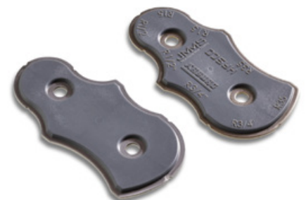
In two mould cavities of a vertical Allrounder 375 V, metal inserts are overmoulded with plastic to produce radius gauges in a cycle time of approximately 45 seconds. (Photo: ARBURG)
