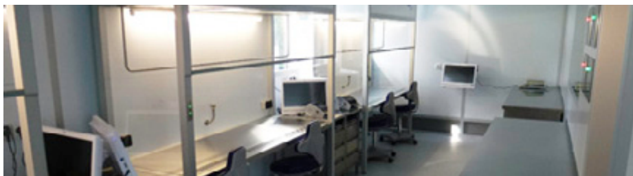
Cleanroom laboratory for parenteral nutrition. CleanSteriCell® GMP A in B with laminar flow workbenches.
