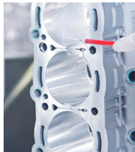
Figure 4: Example of an extraction by means of pressure-rinsing
