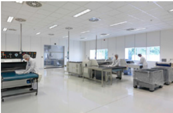
STRUBL cleanroom production ISO 7 for manufacturing of cleanroom packaging
