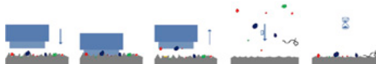
Figure 8: Principle of the Tape Lift method (left) and collecting particles with sedimentation traps (right)
