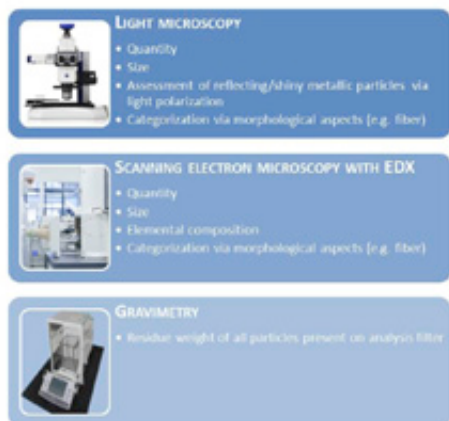
Figure 5: Information obtained from different analysis techniques
