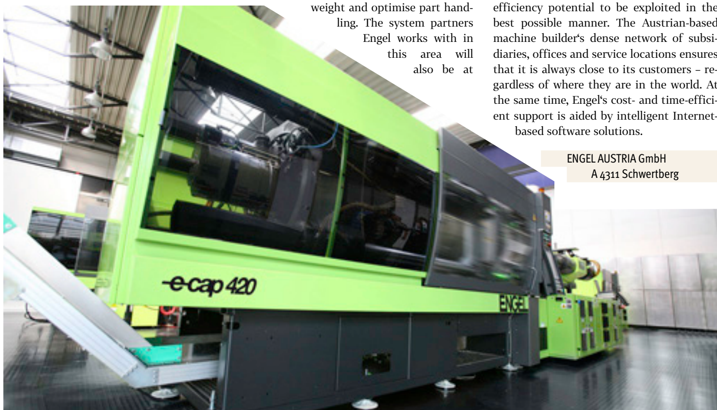
The all-electric Engel e-cap 420 has a clamping force of 420 tonnes and is the largest machine in the high-performance series. It achieves cycle times of less than three seconds.
