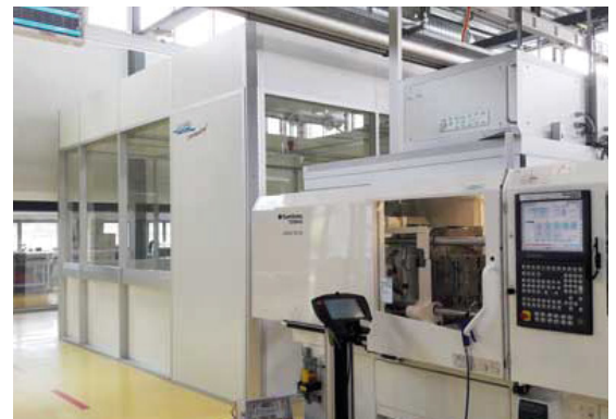
Cleanroom solution with docked injection moulding machine
