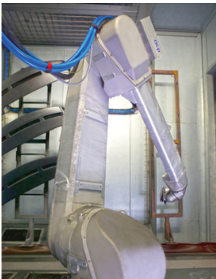
The cleaning process is very similar to the painting process with robots, enabling almost identical programming solutions to be used. (Photo source: acp systems AG)
