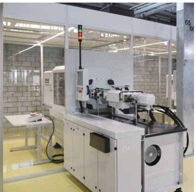
The injection units with the high heat loads remain outside the fully glazed cleanroom
