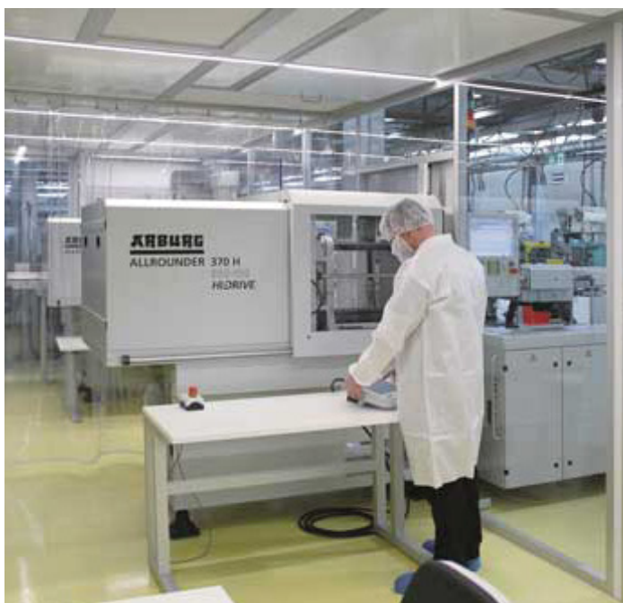
In the cleanroom CleanCell4.0®, the finished parts can be removed directly
