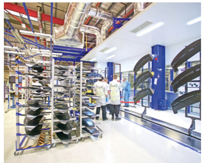
The cleaning process can be easily integrated into the painting line, as well as controlled by a production control system. (Photo source: acp systems AG)
