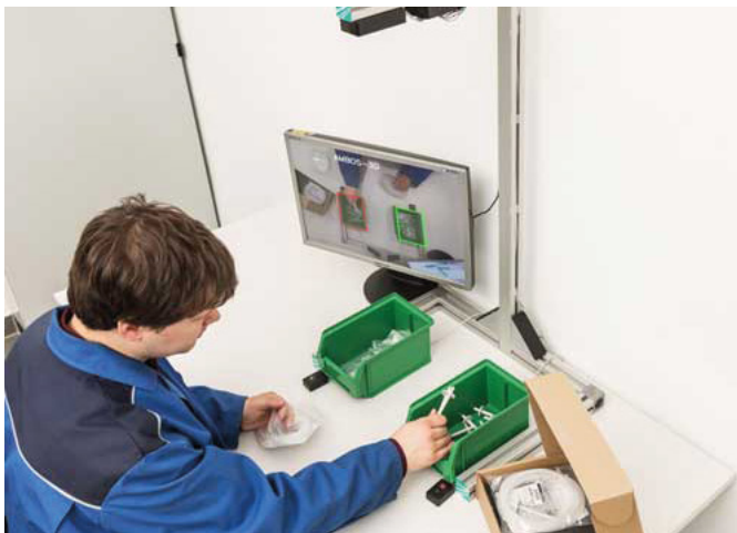
Due to its smart algorithms and powerful 3D sensors, this partially automated assembly assistant system is able to recognize which step of the procedure is under completion and intervene when an error occurs. (© Fraunhofer IPA/Photo: Rainer Bez)
