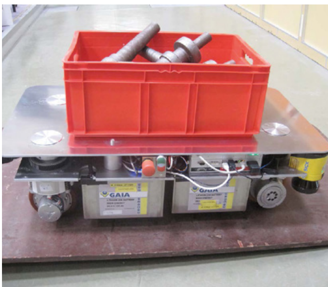
Automated guided vehicles need to position themselves underneath loads in order to pick them up. For this reason, they need to be as flat as possible. The structure of the new omnidirectional drive module above the wheels is therefore very slim. (Photo: Fraunhofer IPA)
