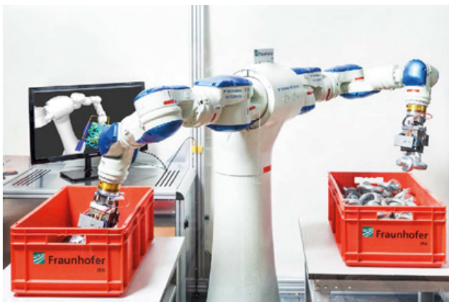
Through machine learning, bin-picking is being further and further refined. In the research project “DeepGrasping“, a virtual learning environment is being created for robots. (Photo: Fraunhofer IPA/Rainer Bez)
