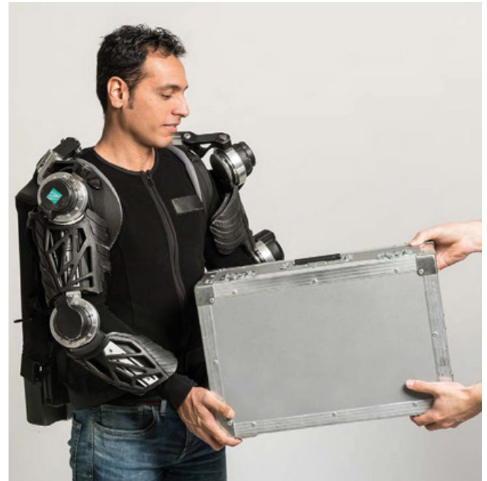
The experts have integrated drive modules at the elbows and shoulders to support high-torque movements. (Photo: Fraunhofer IPA)
