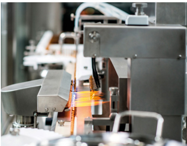
ALF 5000 filling and closing machine: The ALF 5000 from Bosch ensures high process safety. For instance, the ampoule heads are removed sideways during closing, instead of from above. (Picture: Bosch)
