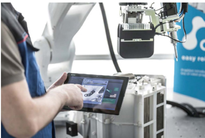
The drag&bot software supplies complete programming modules, which can be put together quickly and intuitively via a graphic user interface to create complex robot applications. (Photo: Fraunhofer IPA/Rainer Bez)
