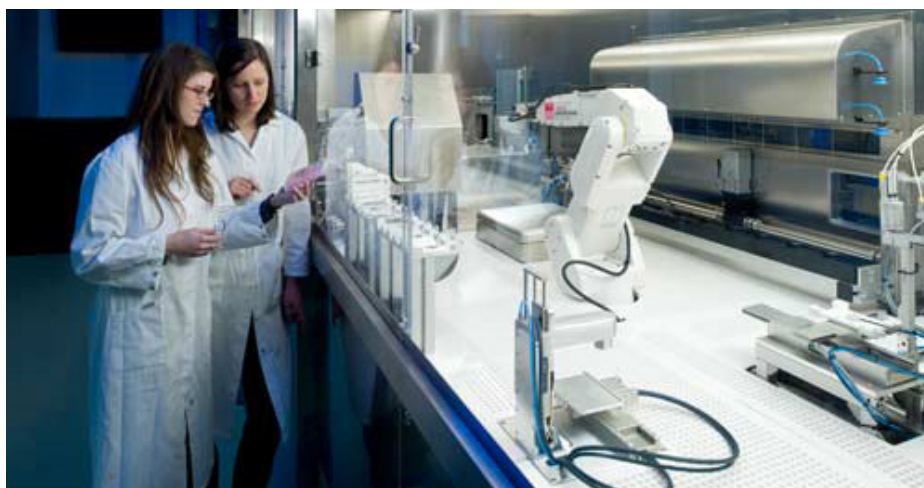
At the Innovation Center nICLAS, members develop technologies for the smart lab of the future. Seen here: automated manufacturing of skin cells at the Tissue Factory.
