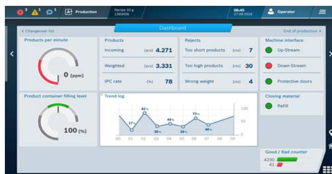
Condition monitoring delivers information on the individual machines or complete lines in real time. Based on pre-defined alarm and failure limits deviations can be detected and eliminated early on. (Photo: Bosch Packaging Technology)
