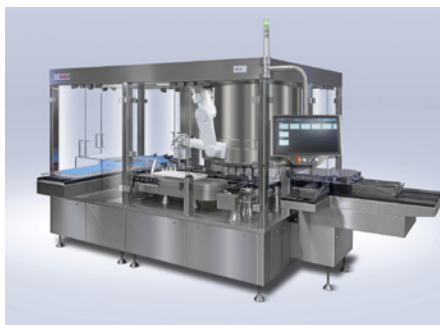
New KLV series for leak detection of rigid glass containers: At Interpack 2017, Bosch unveils the first member of the new KLV series – the KLV 1360 for vials. The platform is suited for inspection of up to 600 standing glass containers per minute. (Picture: Bosch)
