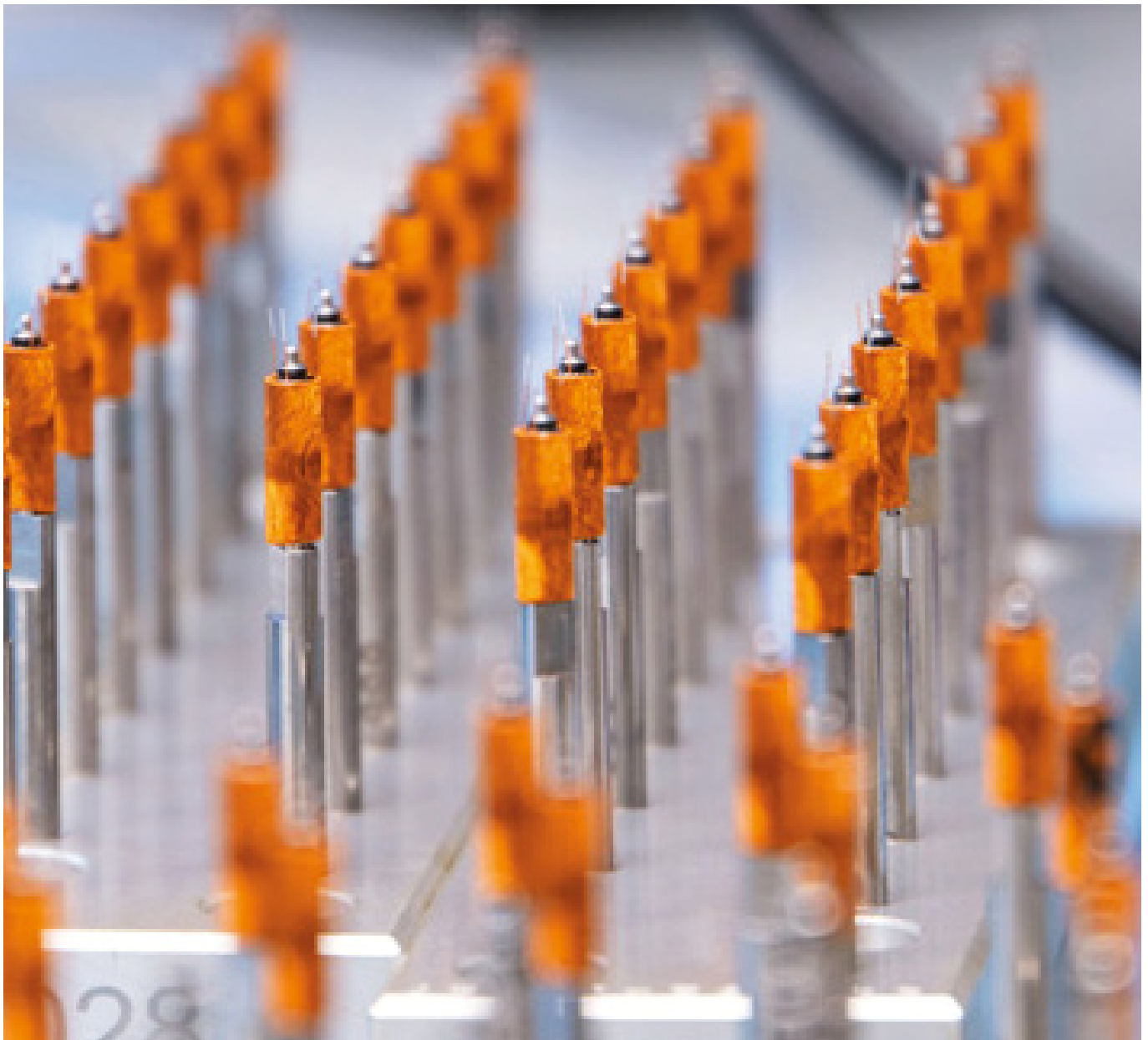
These windings in the cleanroom of maxon in Switzerland are ready for use. They will soon serve in brushless micromotors with a diameter of 6 millimeters. These midgets are in high demand, especially in medical technology. The enameled copper wire has a diameter of less than 0.07 millimeters, about the thickness of a fine human hair.
