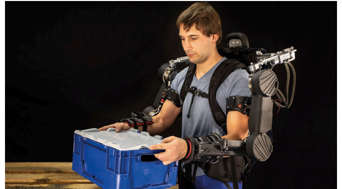
The Stuttgart Exo-Jacket actively supports the upper body during manual handling tasks, in particular during lifting and overhead activities. (© Fraunhofer IPA/Image: Rainer Bez)
