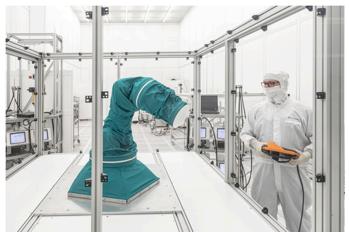
The recently patented 2ndSCIN® protective cover ensures the cleanroom compatibility of any moving automation component. (© Fraunhofer IPA/Image: Rainer Bez)
