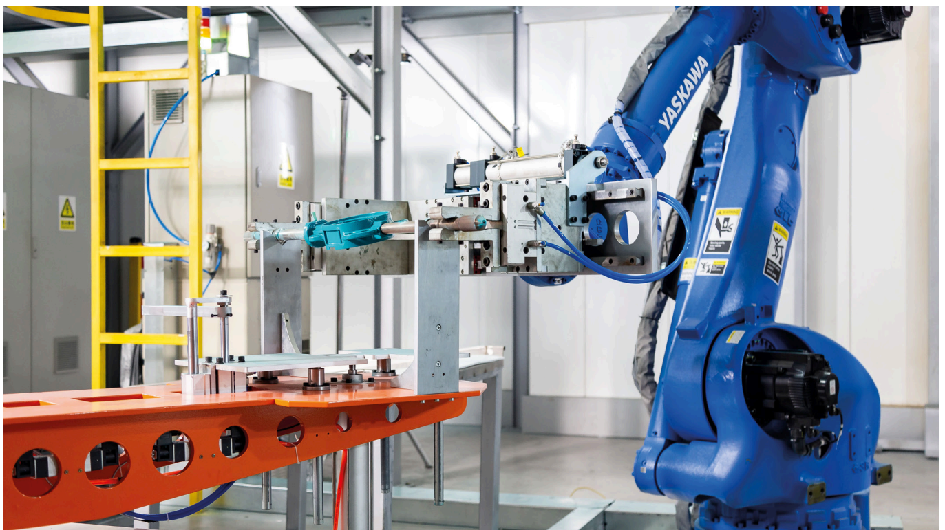
Most modern robot technology in the production process of the GEMÜ R480 butterfly valve.
