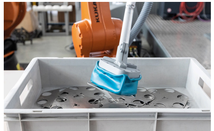
Within the framework of the »Cognitive Robotics« initiative, for example, technologies for machine learning are being further developed for bin picking applications. (© Fraunhofer IPA/Image: Rainer Bez)
