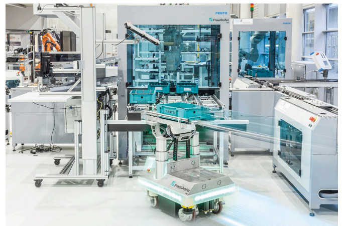
Autonomously navigating mobile robots are a key element for flexible production and logistics applications. (© Fraunhofer IPA/University of Stuttgart IFF Image: R. Bez)
