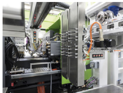
When producing pipette tips, the unhindered access to the mould area of the e-victory injection moulding machine allows for an especially close fitting of the automation to the clamping unit. (Picture: Engel)
