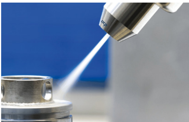
The CO 2 snow jet technology selectively dry-cleans specific areas of components without leaving any residues, for example before or after laser-welding processes. (Photo: acp – advanced clean production)
