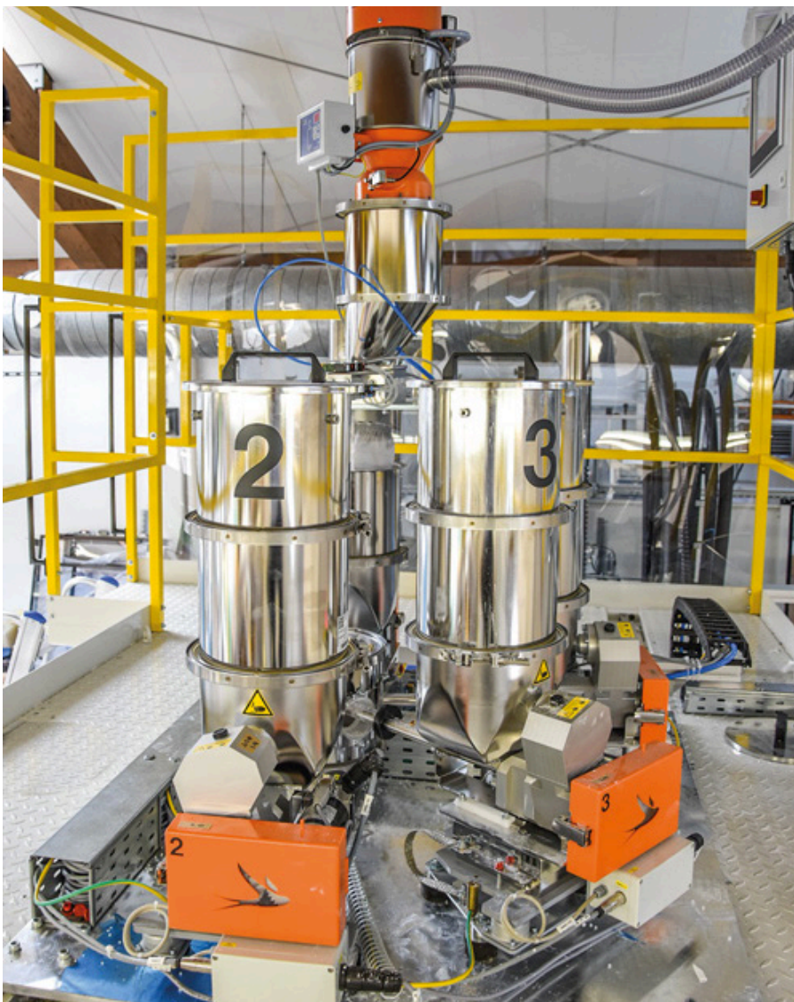
The modular dosing system comes with four different dosing modules and can be quickly and easily adapted for feeding granulate, micro granulate, powder, grinding stock and liquids and various dosing tasks. (Image: motan-colortronic)
