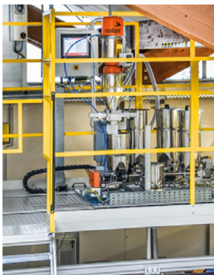
Graviplus-series gravimetric synchronous dosing and blending station with four Labline dosing modules, one of which can be automatically supplied with material by a Metro conveying unit, while the other three have to be manually filled. (Image: motan-colortronic)
