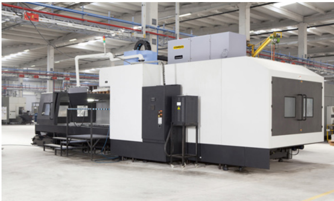
Fig. 1: Modern CNC cutting machines increase the amount of contaminants in the air in factory buildings; this can be remedied by air purifiers. (Photo: ISI-Industrieprodukte GmbH)
