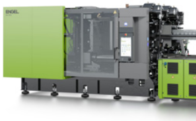
New horizons for the automotive industry: At Fakuma, for the first time ENGEL will be producing exterior components on a duo 500 injection moulding machine using the clearmelt process. (Picture: ENGEL)
