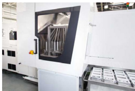
Compact integration: The pipe distributor fits in the machine's safety guard. (Picture: ENGEL)
