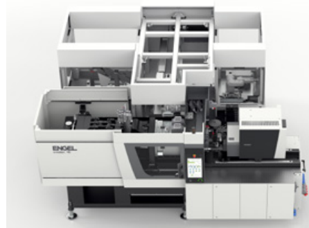
The production technology developed by ENGEL in cooperation with Hack Formenbau and Hekuma makes it possible to fully form up to 500 bristles using a single-component process. (Picture: ENGEL)
