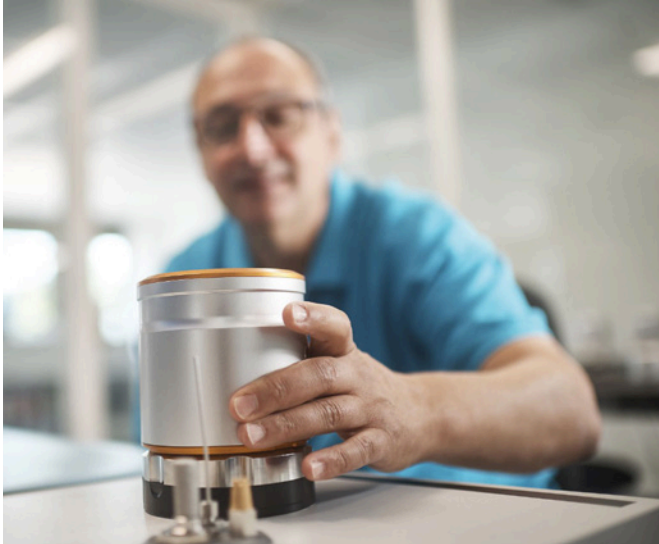
A DA-100 NT digital anemometer for the calibration of the air flow of MAS-100 air samplers is tested in the ISO 17025 accredited calibration laboratory of MBV.
