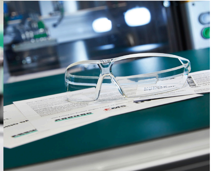
In April, a trade fair demonstrator became an application for safety goggles – distributed to nursing and medical staff during the corona pandemic. The glasses are manufactured on a turnkey system around an electric Allrounder 570 A. (Photo: Arburg)
