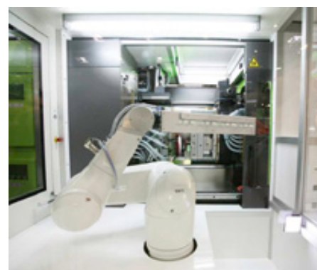
Reliable production processes are necessary for the manufacture of medical devices under cleanroom conditions. An injection moulding cell produced by Engel with fully integrated Stäubli cleanroom robot readily complies with all the relevant requirements. Photo: Engel
