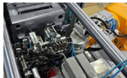
A Stäubli RX160 scores in terms of maximum precision whilst carrying out insertion / removal operations on injection moulds. Yet at the same time, movement sequences must be extremely rapid in order to keep tool-open times as short as possible.
