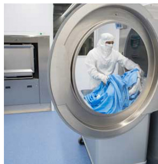
The employees have been specially trained for safe conduct inside the cleanroom. Here you can see the dryer unloading process.
