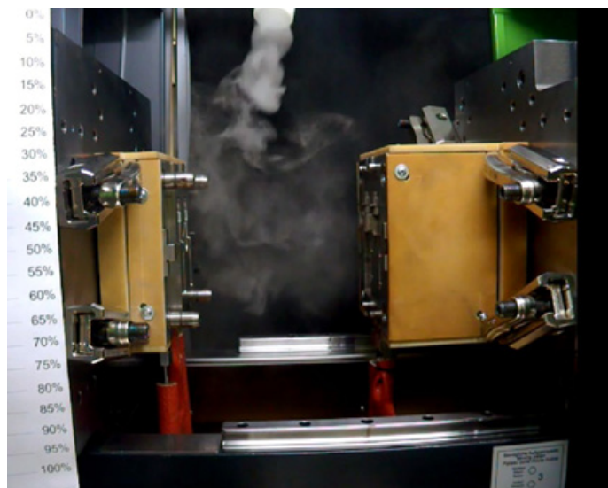
Figure 3. At a mold temperature of 140°C, it was only possible to achieve a throughflow by increasing the flow velocity, which, however, is not permitted in practice due to the fixed velocity of 0.45 m/s. (Picture: ENGEL)
