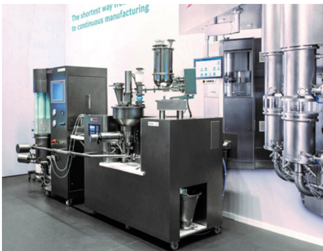
Xelum R&D by Bosch: The R&D device for the production of oral solid dosage (OSD) forms ensures short time to market and an optimum dosing of smallest amounts of API.
