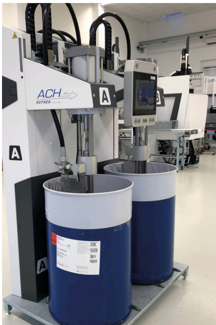
A MaxiMix G2 from ACH-Solution is used for metering the liquid silicone rubber. The entire process can be conveniently controlled via the CC300 operating panel of the ENGEL injection moulding machine. (Picture: ACH-Solution)
