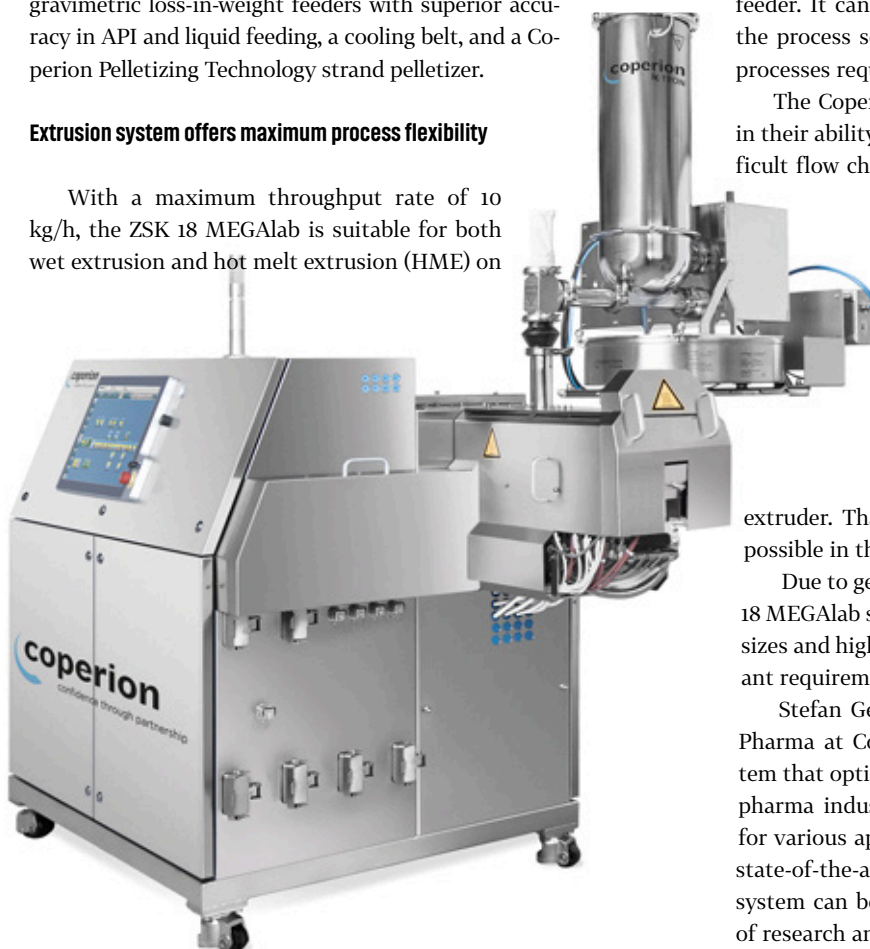
Coperion's ZSK 18 MEGAlab twin screw extruder with Coperion K-Tron gravimetric loss-in-weight feeder, suitable for research and development as well as for small-scale production. (Photo: Coperion, Stuttgart)
