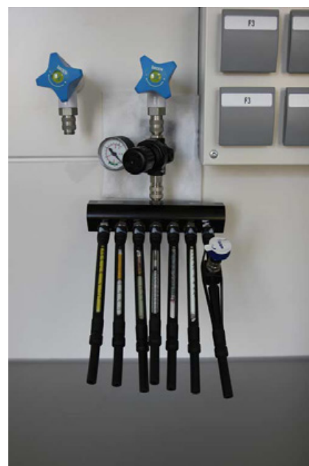
Fig. 6: Visual inspection of low trace gases via oil impactor
