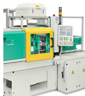
Special micro production cell: An electric Allrounder 270 A, the new micro injection unit and a Multilift H 3+1 robotic system form a flexible system solution for the manufacture of micro components. (Photo: Arburg)
