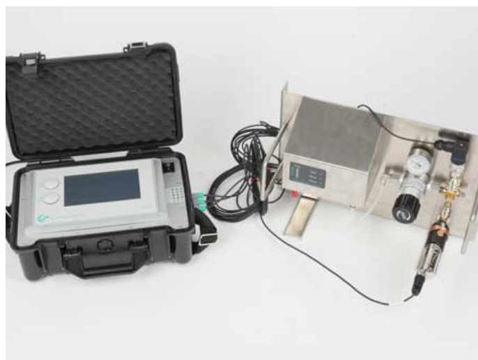
Fig. 2: Measurement system for the determination of the particle content
