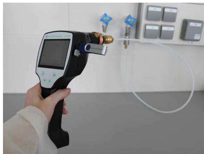
Fig. 3: Test of the pressure dew point
