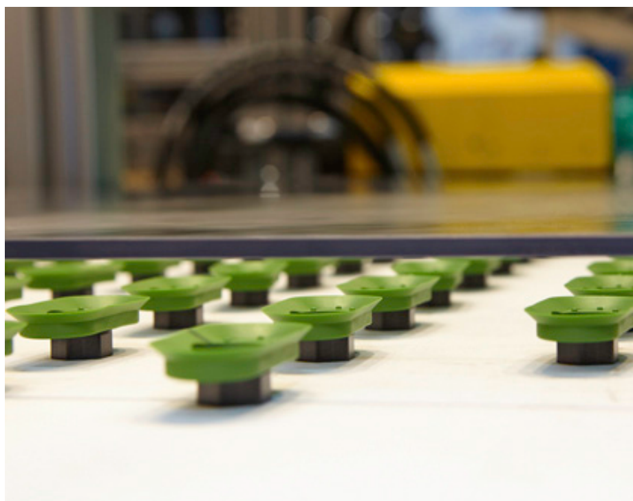
Production process with know-how: complete suction pads can be produced from LSR and thermoplastic in a single operation. (Photo: Arburg)
