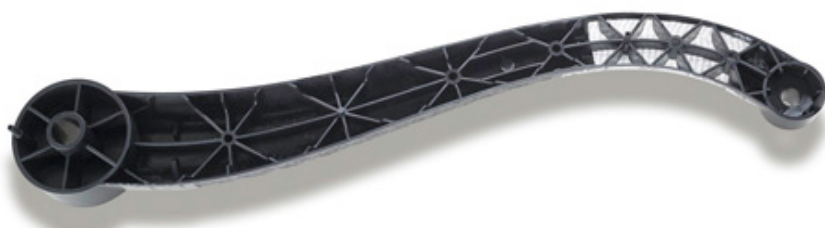
Arburg is presenting the innovative long-fibre direct injection moulding process at the NPE 2015 with an energy-optimised hydraulic Allrounder 820 S in combination with the overmoulding of a continuous-fibre reinforced thermoplastic insert (organic sheet). The composite part weighs only around 200 grams at a length exceeding 500 millimetres. (Photo: Arburg)
