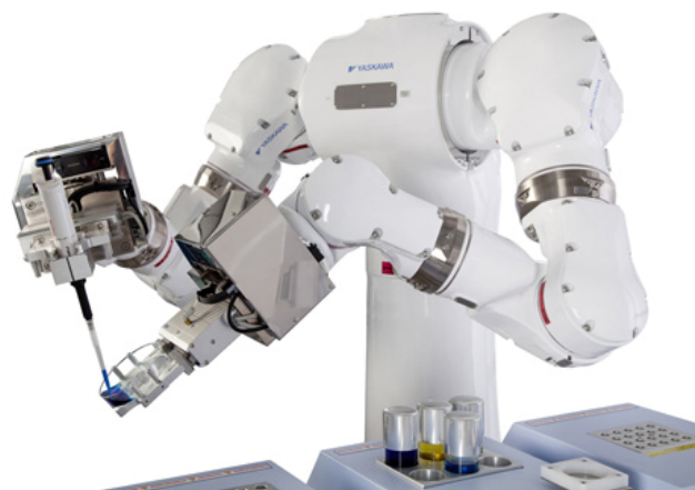
The Yaskawa dual-arm robot, shown here in action in the laboratory, is now revolutionizing the testing of medical diagnostic devices. (Photo: Yaskawa)
