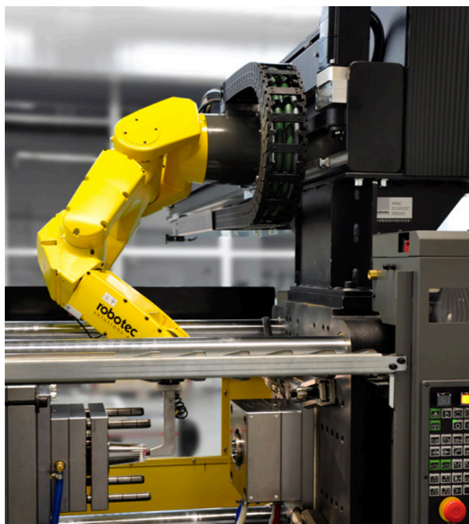
The traversing axis driven by a Fanuc servo motor gives the robot additional range. (Photo: Robotec Solution)
