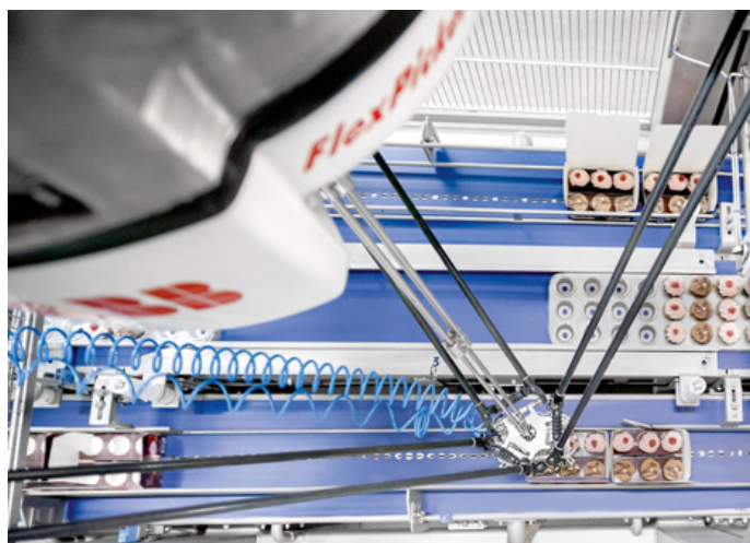
Delta robots such as the legendary ABB FlexPicker have proven themselves both in secondary and primary food packaging. (Photo: ABB)
