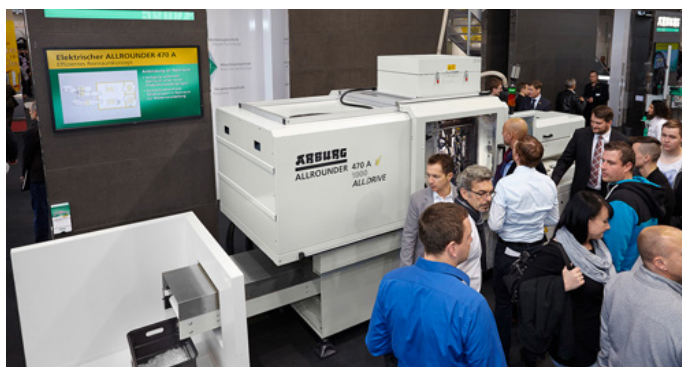
At the Medtec Europe 2016, an electric Allrounder 470 A will use a Männer mould to produce eight Y-connectors for use in intravenous drip therapy in a cycle time of around 12 seconds. (Photo: ARBURG)
