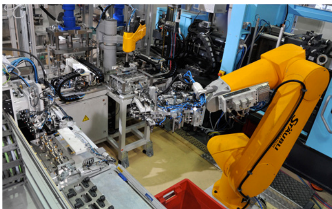
The automotive supplier TRW relies on complete machining of sophisticated plastic parts directly on injection molding machines. (Photo: Ralf Högel)
