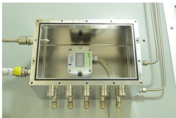
Figure 2: The devices under calibration are placed in a chamber with precisely defined gas concentration. (Photo: E+E Elektronik Ges.m.b.H.)
