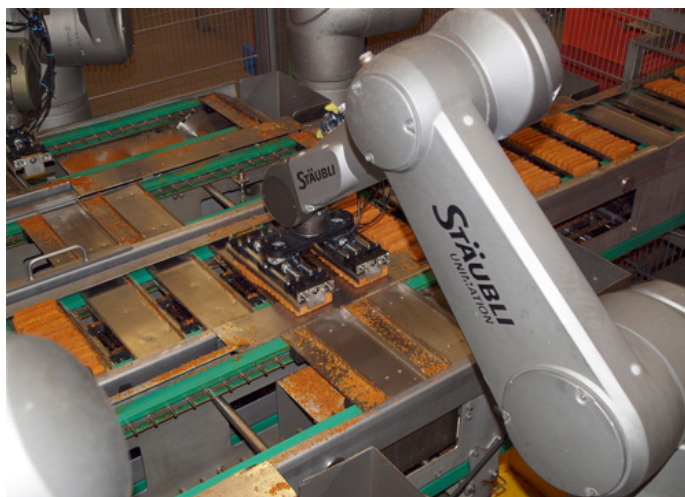
The encapsulated Stäubli robots in HE design have no problems dealing with crumbly fish sticks and daily cleaning cycles. (Photo: Winkler)
