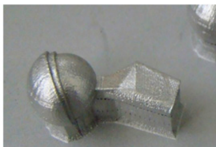
Active quality assurance using QMmeltpool: although the human eye is incapable of detecting defects, QMmeltpool nevertheless identifies deviations in component quality. (Photo: Concept Laser GmbH)
