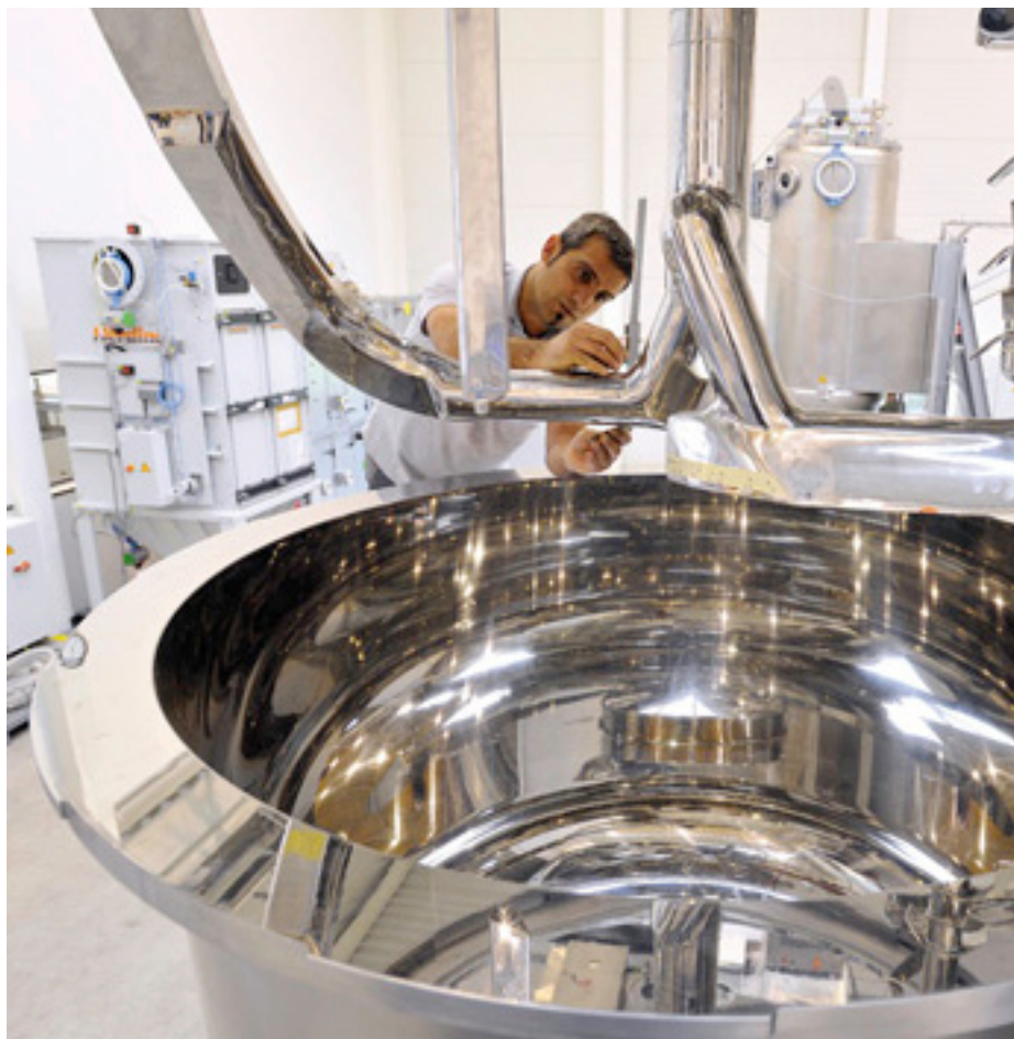
Hüttlin Gentlewing: Thanks to its special geometry, the Hüttlin Gentlewing mixing device by Bosch Packaging Technology achieves maximum mixing quality while exerting low mechanical stress on the product.
