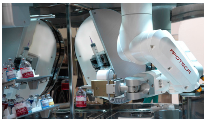
The TX40 CR (cleanroom) robot takes on the job of preparing toxic compounds for chemotherapy.
