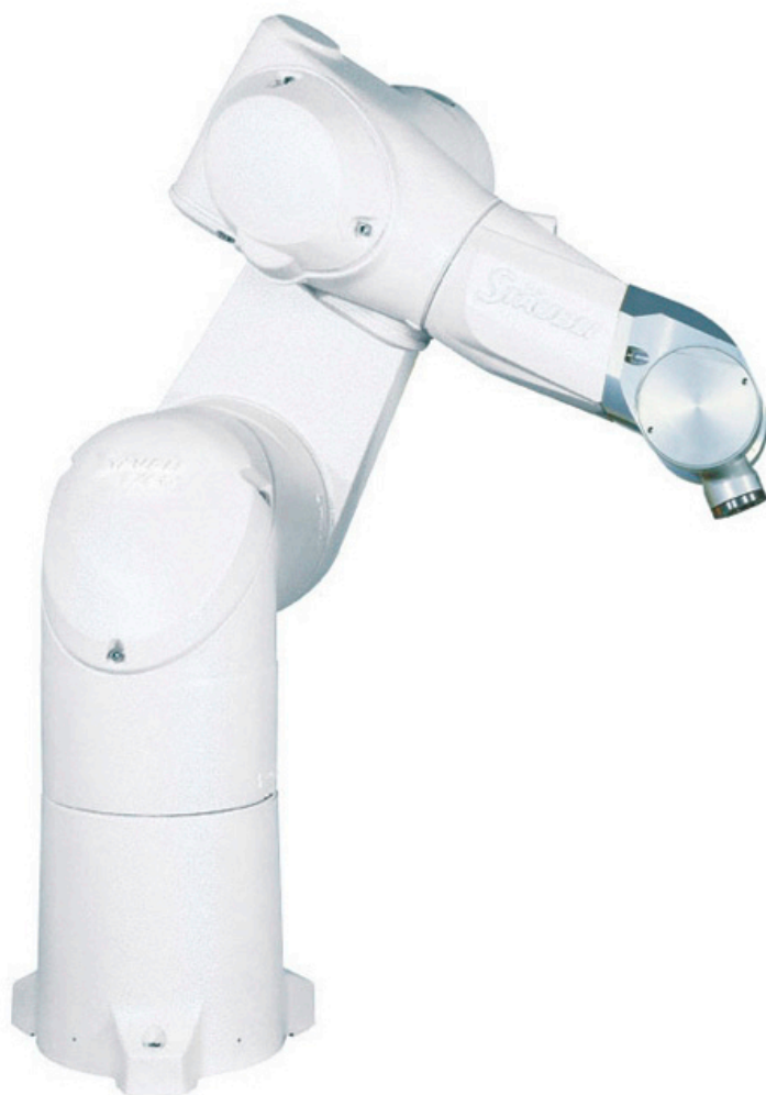
The CR versions of Stäubli cleanroom robots comply with ISO Class 4, while the SCR versions satisfy ISO Class 2-3.
