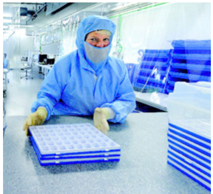
In this area, people are obliged to wear masks: staff members assemble and package products under class 7 cleanroom conditions – the products must be kept free of contamination from hair or dust. (Photo by thinXXS)
