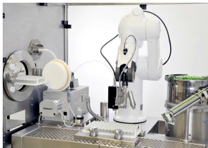
The TX60 Stericlean is responsible for the aseptic pipetting of pharmaceutical products. The production unit fills as many as 600 vials per hour.
