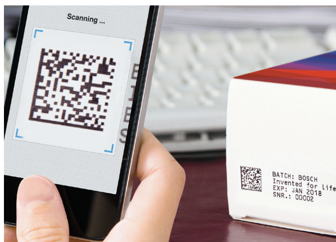
Industry 4.0: Track & Trace: The CPS (Carton Printing System) forms the basis of all serialization solutions from Bosch. The printer can be flexibly adjusted, either to print the data matrix codes on top or on the side of the folded cartons. The new CPI Software from Bosch ensures reliable connection between software and machine level during the serialization process.
