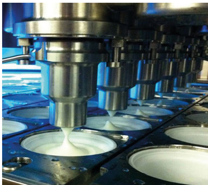
Osgood Industries Inc.: Osgood Industries Inc, Florida, develops, manufactures and distributes Fill- and seal equipment for pre-formed containers in the liquid food industry. Pictured is a fill- and seal machine for yogurt.
