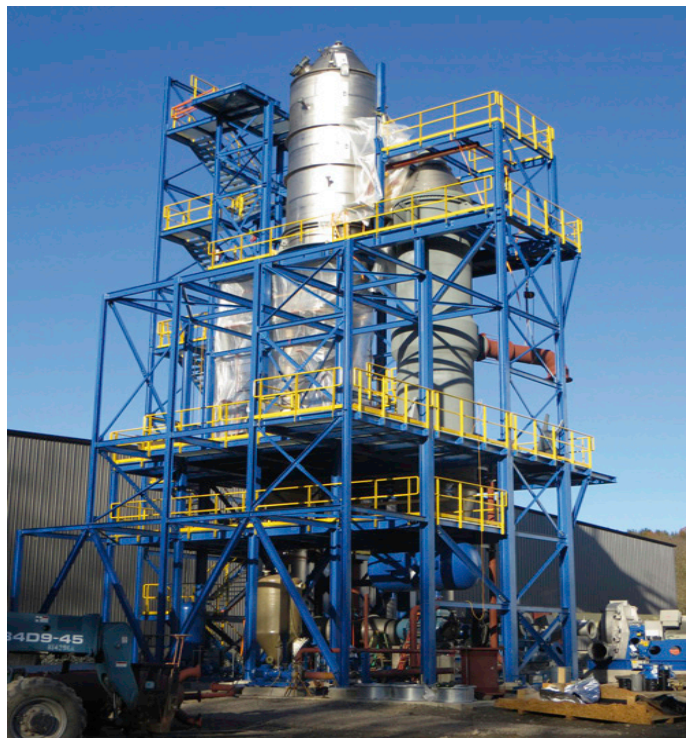
Example of an evaporation unit forming part of a ZLD process.
