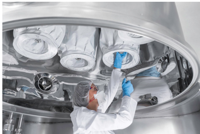
Crucial for high yields: the process filters: To obtain high yields in the fluid bed module of the new GranuLean, Bosch has developed a new process filter.
