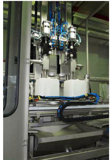
The SMB filling system cubicle is made entirely out of stainless steel. Up to 200 canisters can be filled in the facility per hour. (Photo: SMB)
