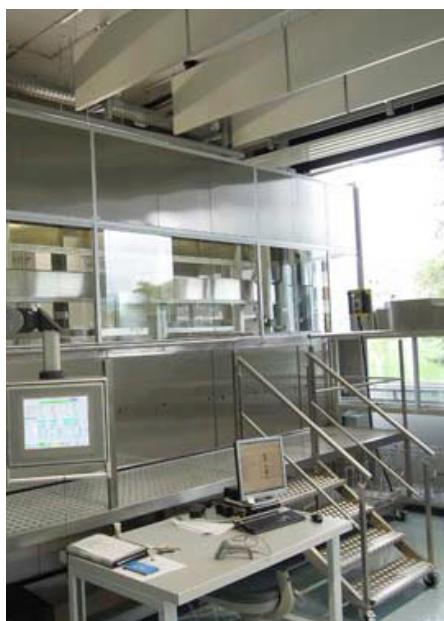
The equipment has a throughput capacity of 12 loads per hour. Part-specific programs are selected by means of a bar code reader (table). (Image source: UCM)
