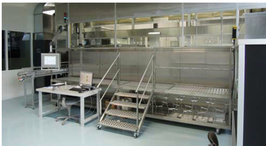
The compact system for ultra-fine cleaning of optical parts and lenses is fully enclosed and comprises eight tanks. (Image source: UCM)
