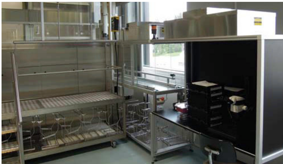
After the cleaning process, a fully enclosed discharge conveyor equipped with a Flow Box delivers the lenses to a quality control station where they are inspected under cleanroom conditions. (Image source: UCM)
