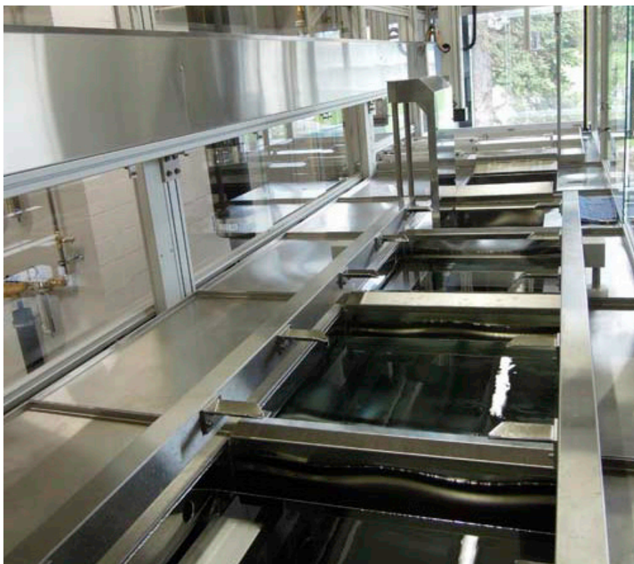
The last two tanks are reserved to HFE drying and are covered with a lid. Parts can be transferred from one tank to the other without removing the lids. (Image source: UCM)
