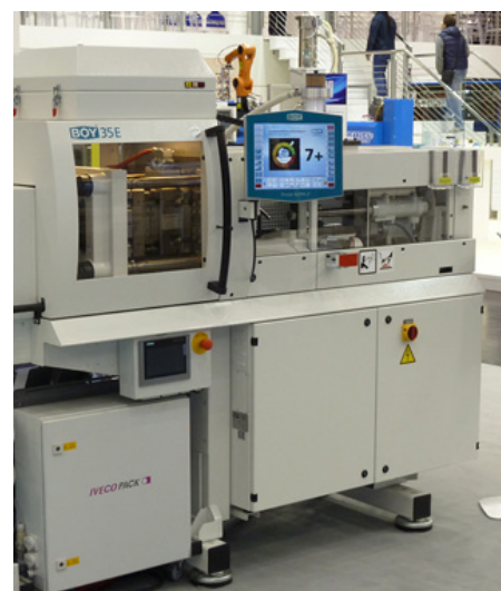
Compact cleanroom application on the BOY 35 E
