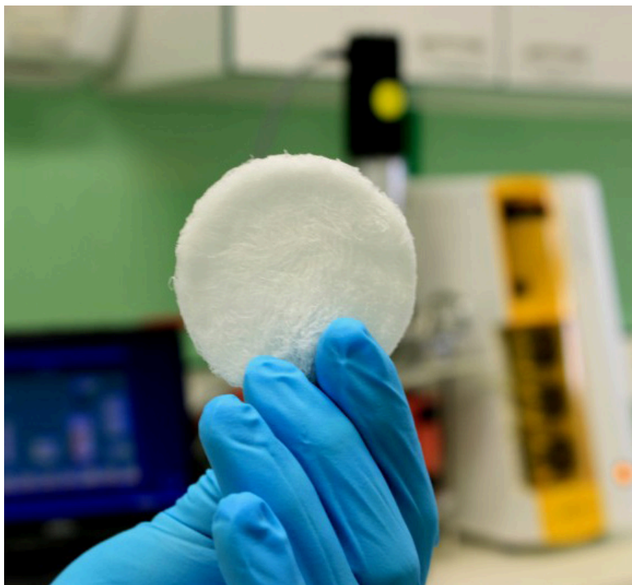
Fig. 2: Wound dressing (nonwoven/fleece) made from alginate fibres derived from bacteria. Bacterial alginate nonwoven materials absorb up to 70% more liquid than marine alginate nonwovens. © Hohenstein Institute
